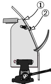
**NOTE:** Start weld on standard and move to SS tube. (It is not necessary to use SS welding rod).
